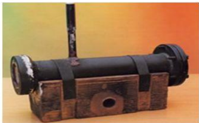
Chadwick's neutron chamber containing parallel disks of radioactive polonium and beryllium. Radiation is emitted from an aluminium window at the chamber's end
