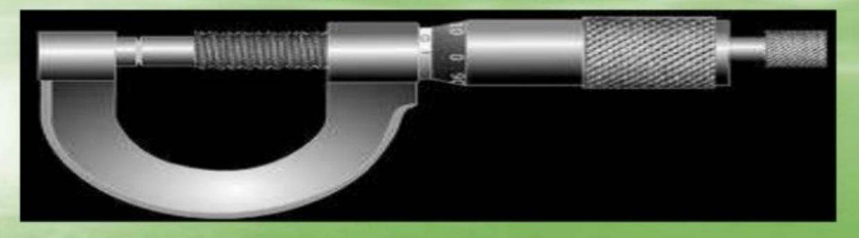
Micrometer screw gauge has a fine threaded movement so that small distances can be measured, with a vernier scale which allows measurement down to thousandths of an inch.
